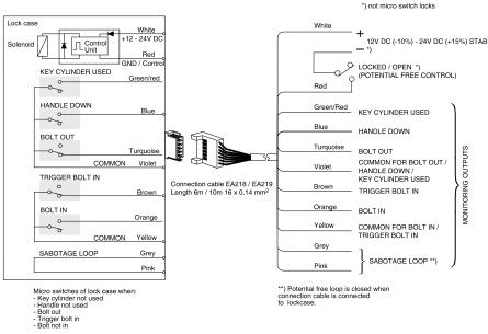
Connector pin-out (cable-side view)
